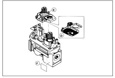
Figure 6.7 Ensure that the rubber gasket (**D**) is properly positioned and install the new HI/LO pressure regulator assembly to the valve using the new screws (**E**) supplied with the kit. Tighten screws securely. (Reference torque = 25 in./lb.) Install the enclosed identification label (**F**) to the valve body where it can be seen.
